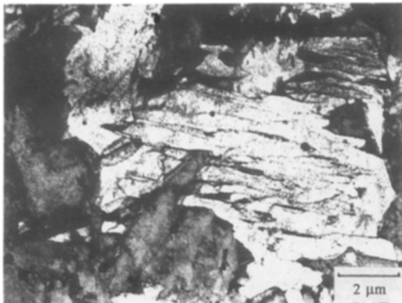
Figure 10 Transmission electron micrograph illustrating the structure in the reheated regions of weld 1.
